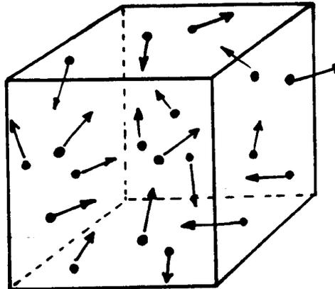
cube with velocity  $v$  and they will make collisions with the nuclei sitting there. We will assume that there are  $N$  nuclei in the  $1 \text{ cm}^3$  cube, and that their absorption ( $n, \gamma$ ) cross-section is  $\sigma_a$ . It turns out that the number of neutrons interacting (ie, being absorbed) per second is given by:
