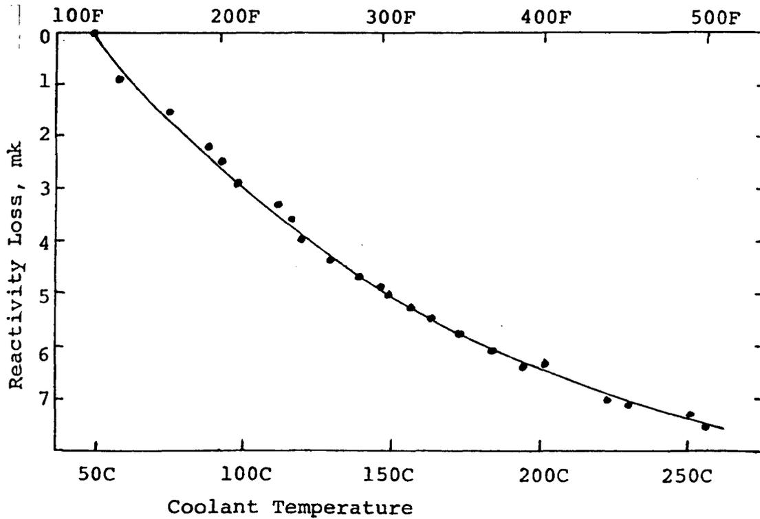
Reactivity Loss Versus Coolant Temperature
