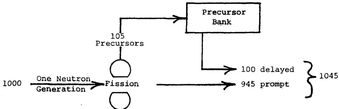
Even though we create 105 precursors we get only 100 delayed neutrons from the precursor bank since it contains precursors produced earlier.
