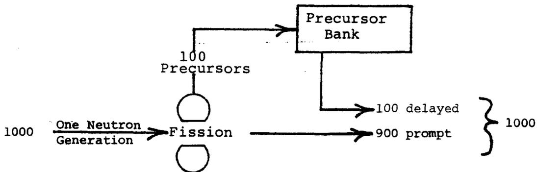
The chain reaction is being maintained at a level of 1000 neutrons per generation. Now insert 50 mk of reactivity such that  $k = 1.05$ :
