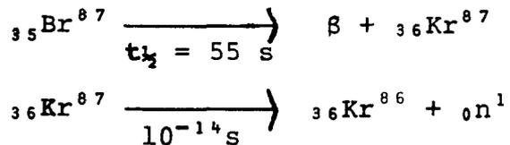
The neutron emission is instantaneous (with respect to Kr-87), but obviously occurs some time after the original fission because the Br-87 must decay first. In fact, it appears to be emitted with the 55 second half-life of Br-87.
