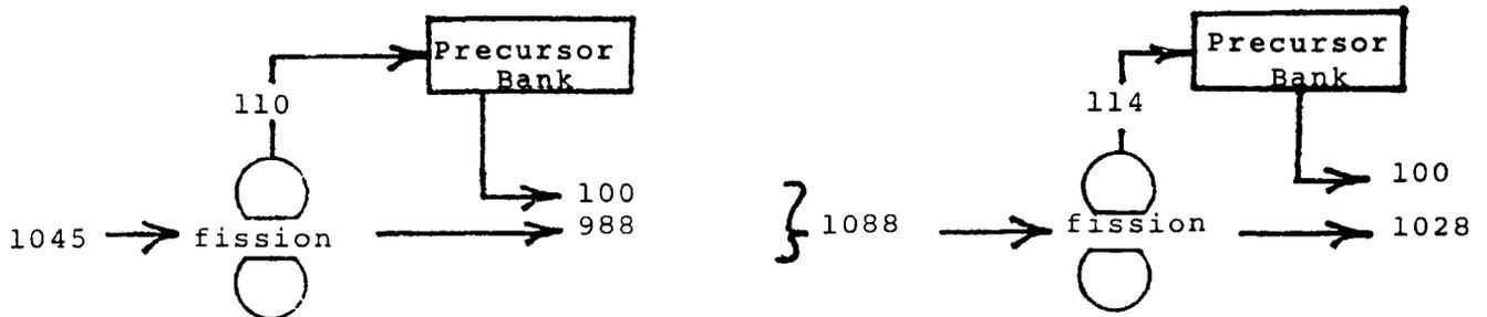
If we assume the output of the precursor bank does not change for a second, we have time for one thousand prompt generations in which time the series will converge to:
