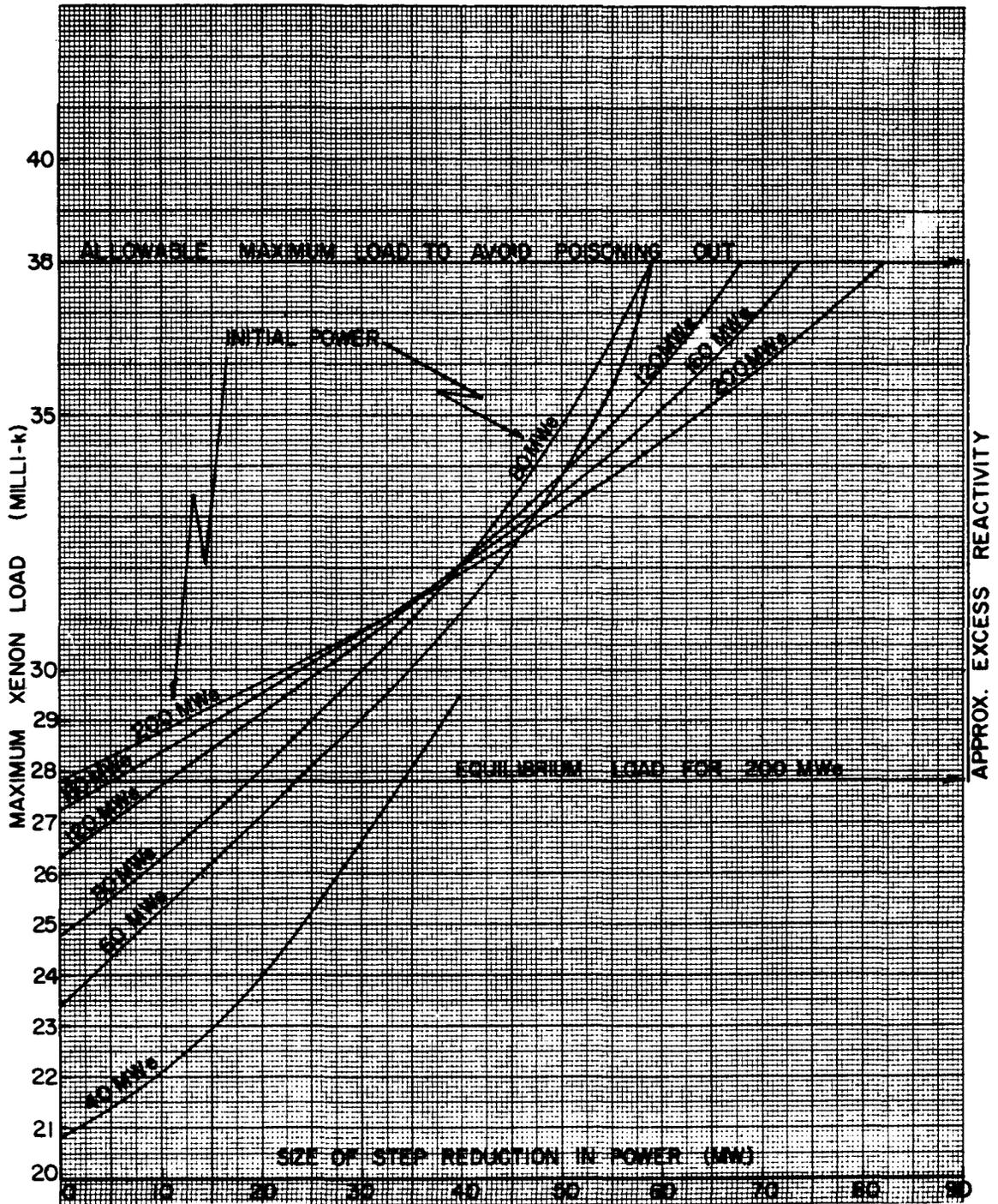
Maximum Xe load attained during the transient following step reductions in power from various initial power levels. (Xenon Assumed to be at the Corresponding Steady State Value Initially; Fuel Assumed to be at Equilibrium Irradiation).
