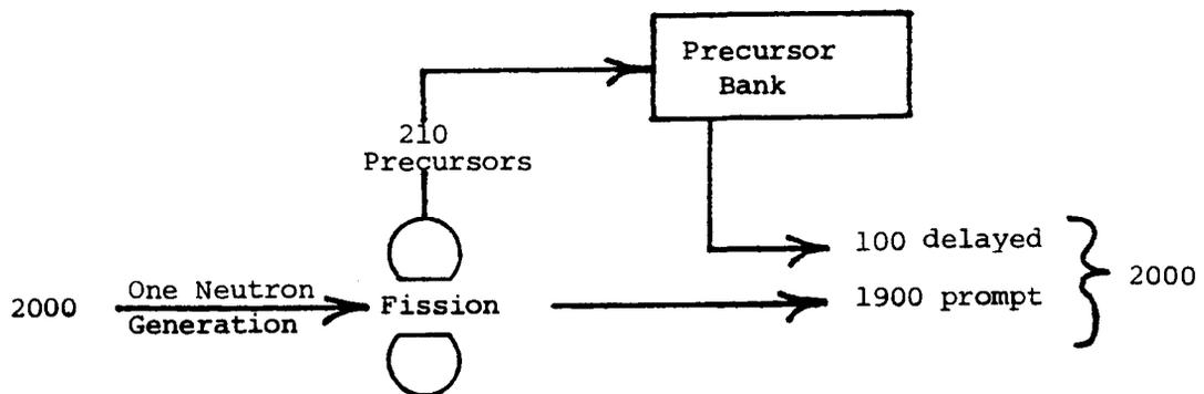
Thus in a very short time period we get a jump in the prompt neutron level but power can not increase beyond a certain point until more precursors start to decay. Therefore, after the prompt jump, the rate of power increase is determined by the decay rate of the delayed neutron precursors. Calculating the magnitude of the prompt jump for this problem using equation (5).
